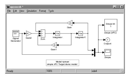
Your next task is to define the xPC Target scope block parameters. See "Defining xPC Target Scope Block Parameters".
