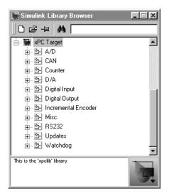
4 Open a function group. For example, to open the A/D group for ComputerBoards, double-click **A/D**, and then double-click **ComputerBoards**.
