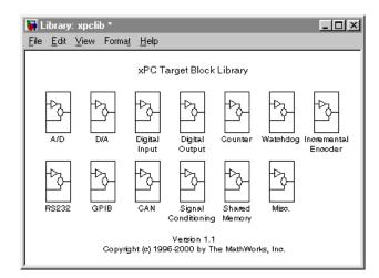
2 Open a function group. For example, to open the A/D group, double-click the A/D block.
