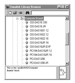
**5** From the block library, click-and-drag the name of an A/D board to the Simulink block diagram. Likewise, click-and-drag the name of a D/A board to your model
