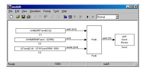
Note that **Port Data Types** and **Signal dimensions** have been turned on from the **Format** menu, showing us that the width of the UDP packet to be sent is 75 bytes. The parameters used in the Pack block are Input port datatypes {'uint8', 'int16', 'double'} and Byte Alignment 1.
