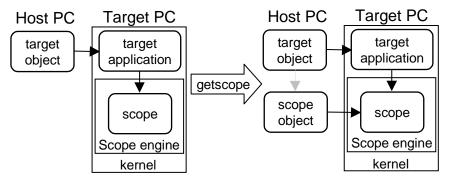
**Examples** If your Simulink model has an xPC Target scope block, a scope of type target is created at the time the target application is downloaded to the target PC. To change the number of samples, you need to create a scope object and then change the scope object property NumSamples.
